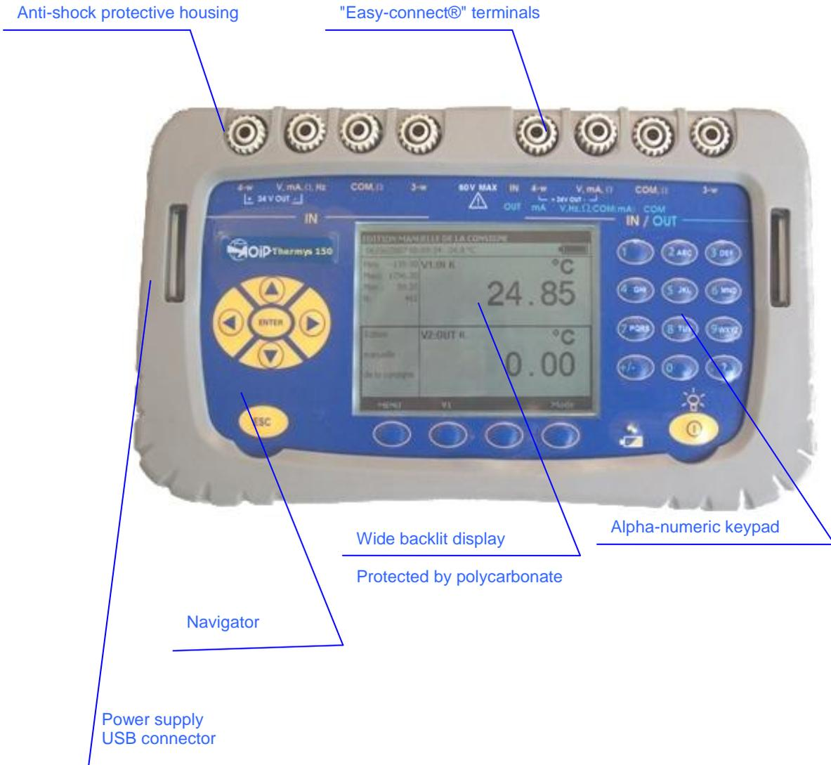
Supplied as standard with a strap and a stand for desktop use, a battery charger and a set of 6 measurement leads with crocodile clips.
